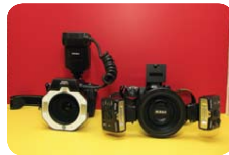
FIGURE 5. Ring flash system on the left, dual-barrel-mounted point flash system on right. The system on the left is heavier and requires more experience.
